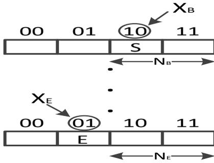
**Figure 5: Position of the first and the last loop instructions in the cache lines**
