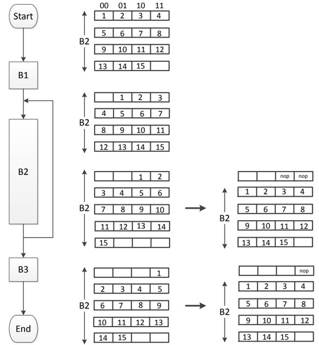
Figure 4: Mapping the B2 loop block into cache lines
