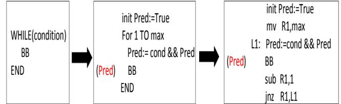
Figure 2: Converted loop code
