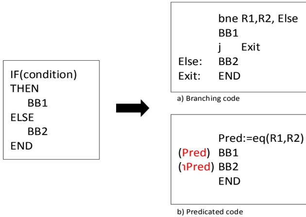
Figure 1: Converted branching code
