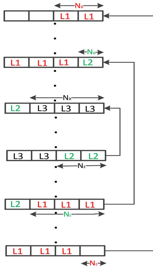
**Figure 6: Nested loops mapped into cache lines**
